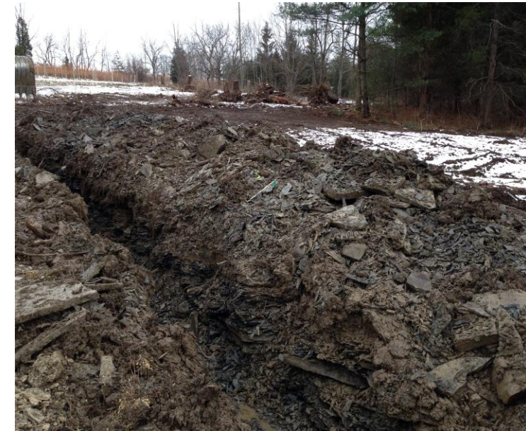
Soil profile of Silver Thread Vineyard block 3 showing very shallow topsoil over shale
